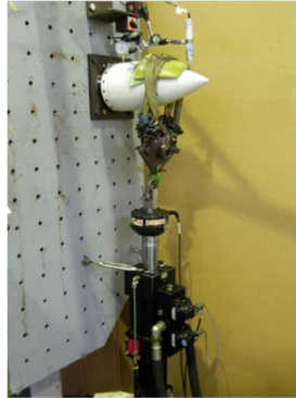
Figure 8: Radome hydraulic pull setup.
